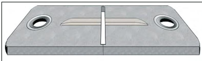
Figure 2. Geradelli's Jig used for the microtensile test.
