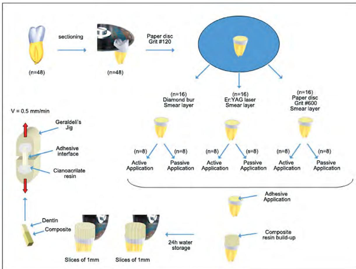
Figure 1. Specimen preparation.
