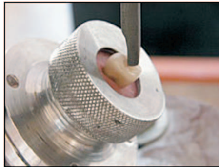
Figure 1. Load application on a specimen tilted at a 45° angle.
