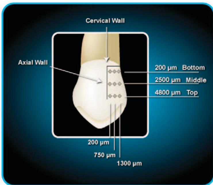
**Figure 2.** Diagram of Vickers indentation location in the internal (200 μm), middle (750 μm), and external (1300 μm) layers in the mesial-distal direction.
