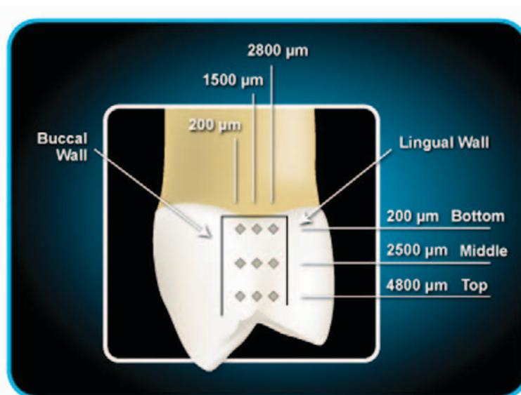
**Figure 1.** Diagram of Vickers indentation location in the proximal surface in the occlusal-gingival direction.
