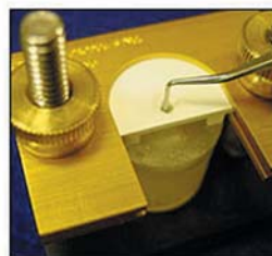
Figure 14. A 1 mm condenser tip is used to press the restorative material into the insert mold below the bevel. Failure to place the material below the bevel will make it impossible to remove the specimen from the mold
