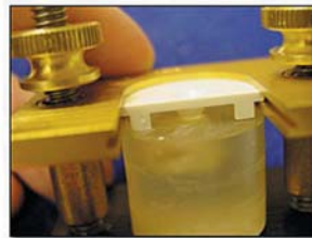
Figure 12. Great care must be taken when positioning and securing the polyethylene bonding mold insert so as not to damage the knife edge.
