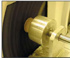
Figure 10. Both ends of the specimen must be ground parallel to each other using coarse and fine grinding wheels. A special rotating grinding apparatus is mounted on a cast trimmer. It should be noted, with unprepared substrates, only the opposite end of the specimen is ground.
