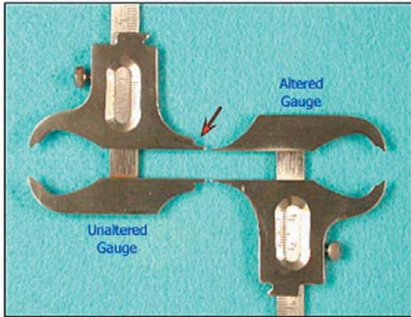
**Figure 1.** Modification of the Boley gauge.
