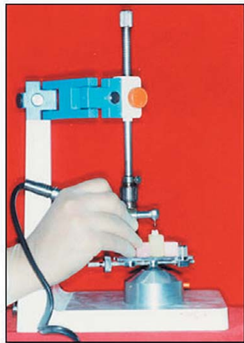
Figure 2. The highspeed handpiece mounted in a surveyor.
