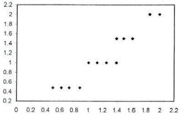
**Figure 7.** Relationship between true and diagnostic depth on Type D film.
