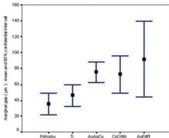
**Figure 2.** Arithmetical mean and confidential interval of the marginal gaps and overextended margins.
