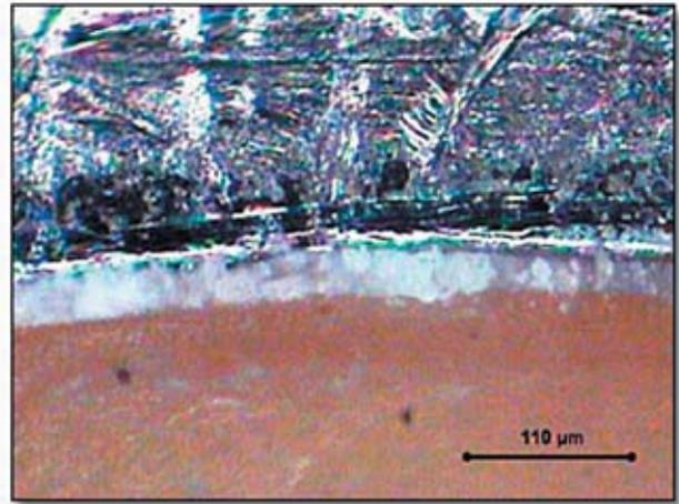
**Figure 4.** Marginal fit of a Ti-cast crown.
