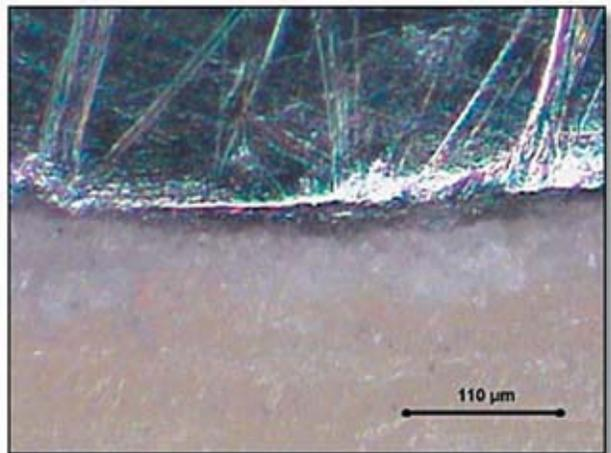
**Figure 8.** Marginal fit of a Ti-milled crown.
