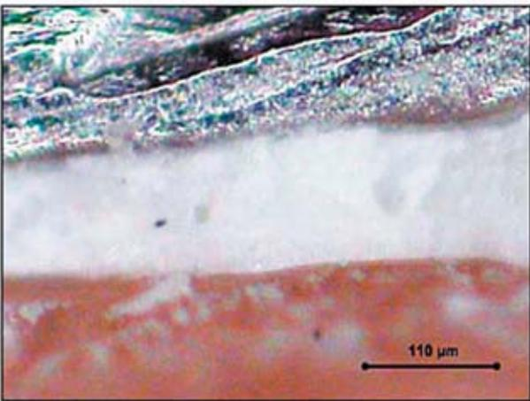
**Figure 7.** Marginal fit of an AuPdPt-crown.
