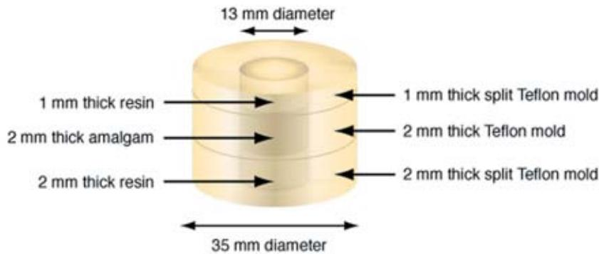
**Figure 1b.** Diagram of the full assembly of amalgam veneered to tooth-colored material for both thickness.
