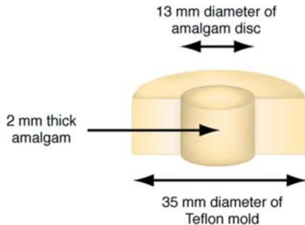
Figure 1a. Diagram of the Teflon mold.
