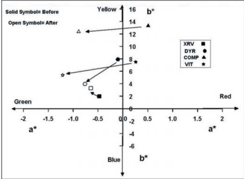
**Figure 3.** The a\* and b\* values of control and resin specimens bonded to amalgam at thickness 2 mm.
