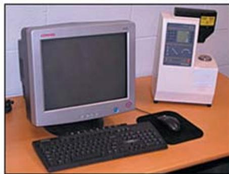
**Figure 3.** Computer setup for use with the Procera<sup>®</sup>, scanning protocol using CAD/CAM technology. (Nobel Biocare USA, Inc., Yorba Linda, CA)
