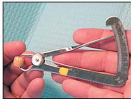
**Figure 6.** Crowns being measured for thickness on the center of the buccal, occlusal, and lingual surfaces.
