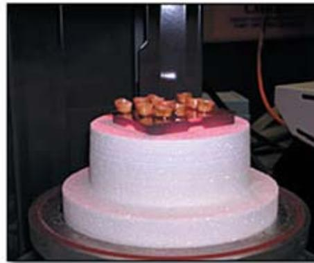
**Figure 4.** Hot Cerac® In-lab copings following glass infiltration process. (Sirona, Charlotte, NC)
