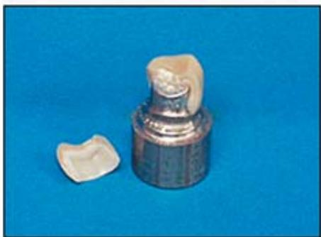
Figure 9. Fractured crown on titanium die.
