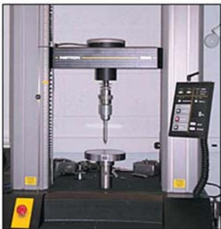
Figure 8. An Instron (Instron Corporation, Canton, MA) universal testing machine.
