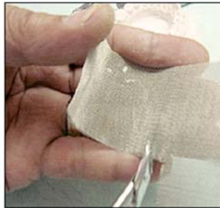
Figure 3. Cutting the metallic mesh to match the outline.
