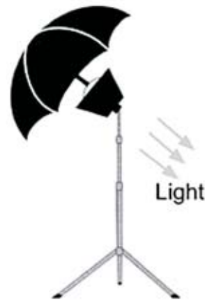
Figure 3. Diagram of a reflective umbrella positioned with the concave side of the umbrella pointed at the subject and the flash is shone on the inside of the umbrella.
