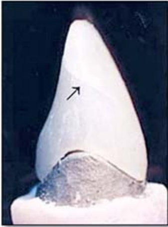
Figure 5. Fracture failure observed in a sample prepared with Protemp II (10X magnification).
