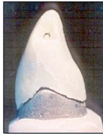
Figure 4. Fracture failure observed in a sample prepared with BISICO Temp S (10X magnification).
