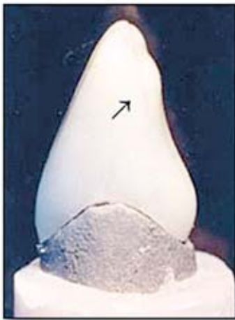
Figure 3. Fracture failure observed in a polycarbonate crown applied fracture load test. Both plastic deformation and cracks were seen in the crown (10X magnification).
