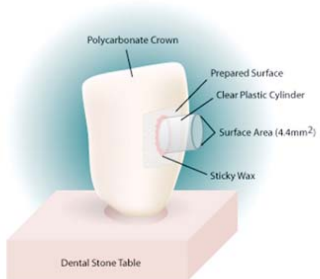
Figure 1. Assembly for shear bond strength testing.
