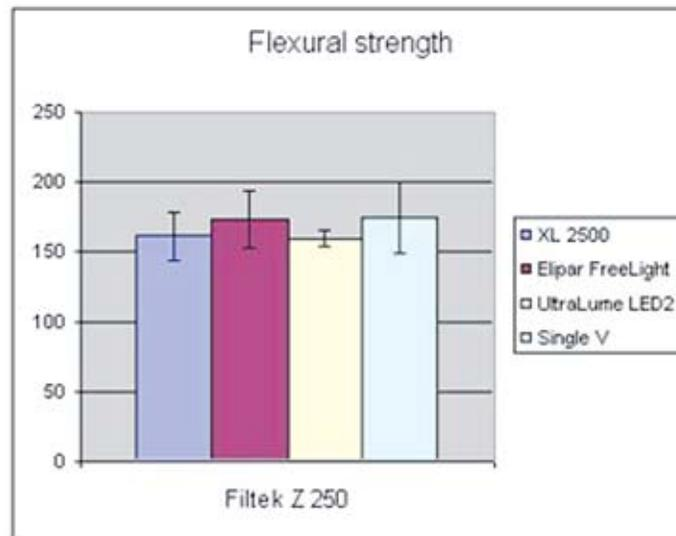
**Figure 3.** Flexural strength of the composite polymerized with the three LED LCUs and the halogen LCU.
