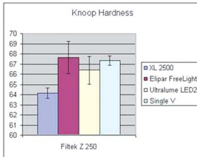
**Figure 1.** Knoop hardness of the composite polymerized with the three LED LCUs and the halogen LCU.
