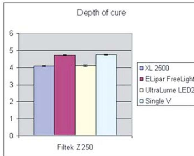
**Figure 2.** Depth of cure of the composite polymerized with the three LED LCUs and the halogen LCU.
