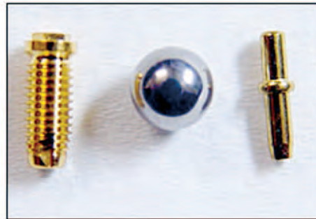
Figure 1. Calibration devices. (a dummy implant, metal ball or any radiopaque metal piece).
