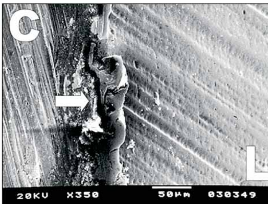
Figure 11. Technique 9 showing an irregular cutting angle and non functional wire edges (arrow) between the coronal (C) and the lateral face (L).
