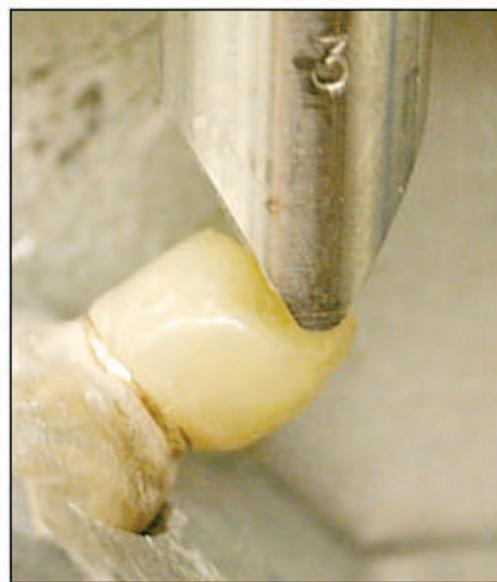
**Figure 1.** Position of loading tip on the temporary crown and the compressive load test setup.
