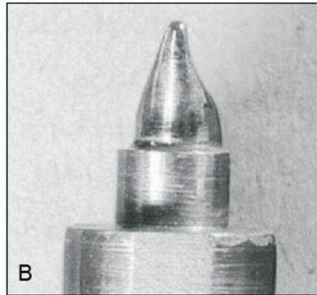
**Figure 2.** The graphical views with detailed dimensions of the dies (A) and Ni-Cr dies (B) used in Group C.
