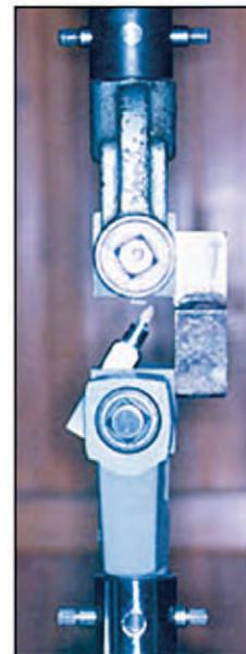
**Figure 4.** Showing the universal testing machine including the Ni-Cr die cemented to the all-ceramic crown and the application of the load.
