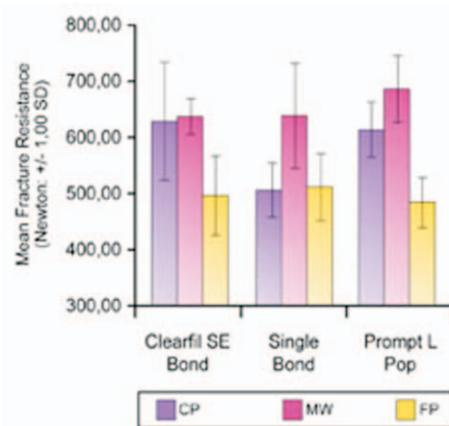
**Figure 1.** The effects of posts and adhesives on fracture resistance.
