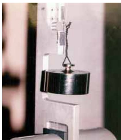
Fig. 3: Mounted jig with bracket archwire and suspended weight
