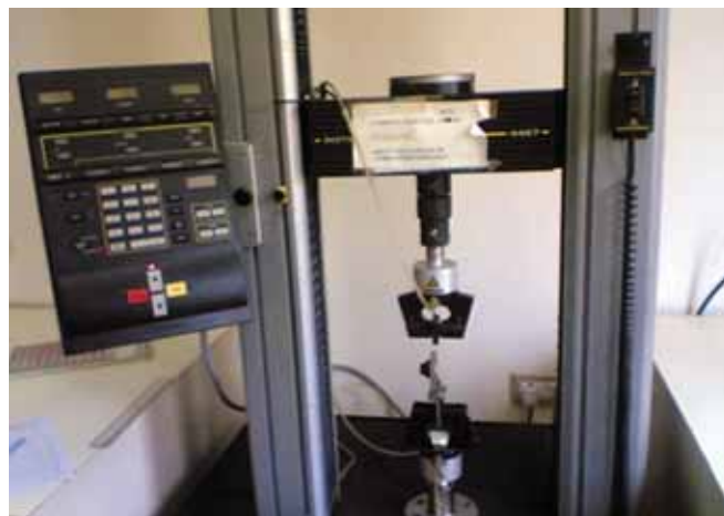
Fig. 5: Instron universal testing machine (model no. 4667)
