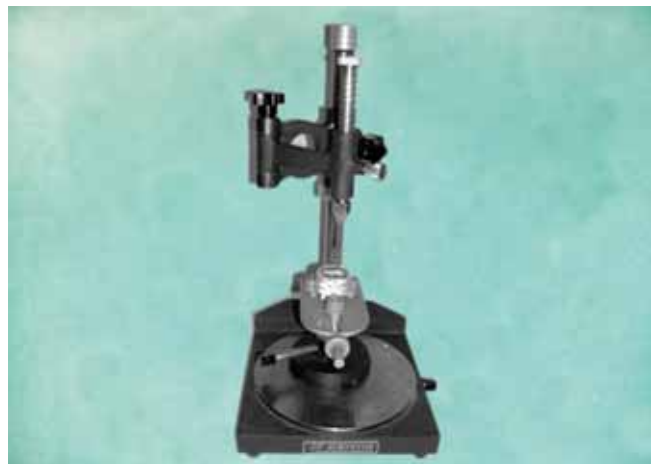
Fig. 1: Surveyor assembly to check the parallelism
