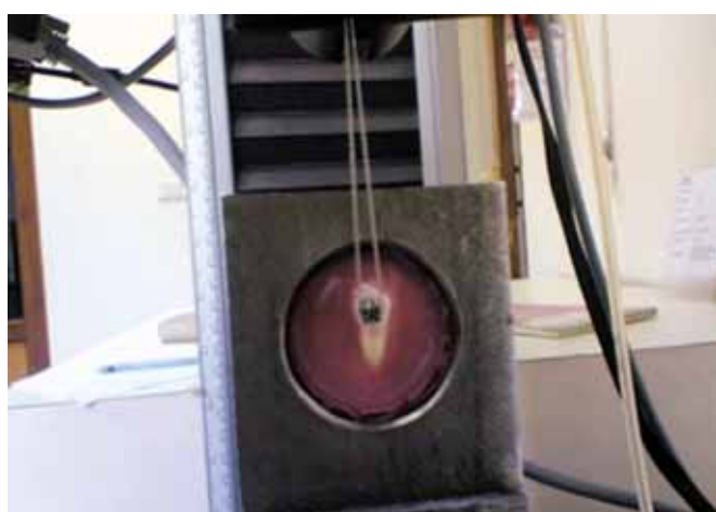
Fig. 7: Specimen mounted for shear bond strength testing on Instron machine
