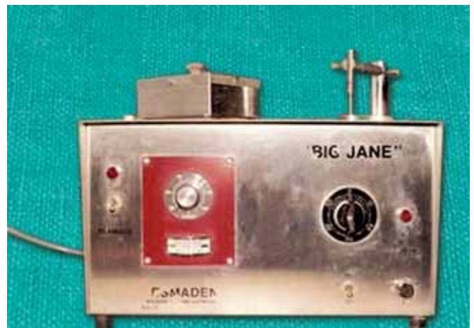
Fig. 3: Recycling unit "Big Jane". Esmadent bracket and band reconditioner
