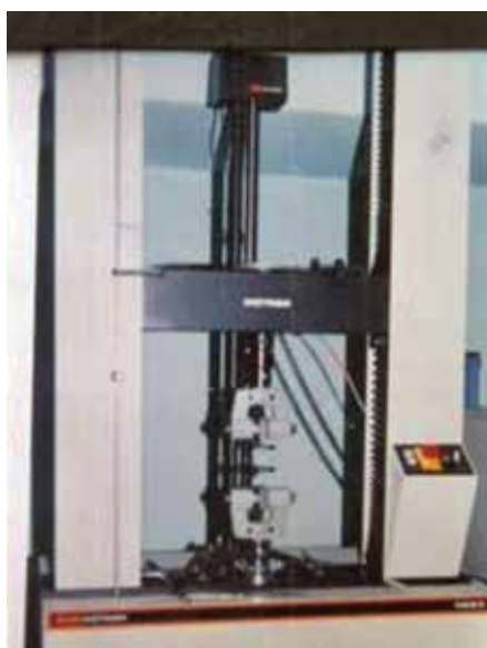
Fig. 7: Acrylic blocks are placed in between the grips of Instron machine for measuring the tensile and shear bond strengths
