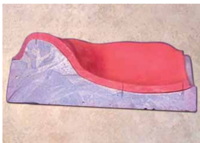
Fig. 18: Reference marks in the processed denture base in anterior, middle and posterior regions after sectioning anteroposteriorly in the midline
