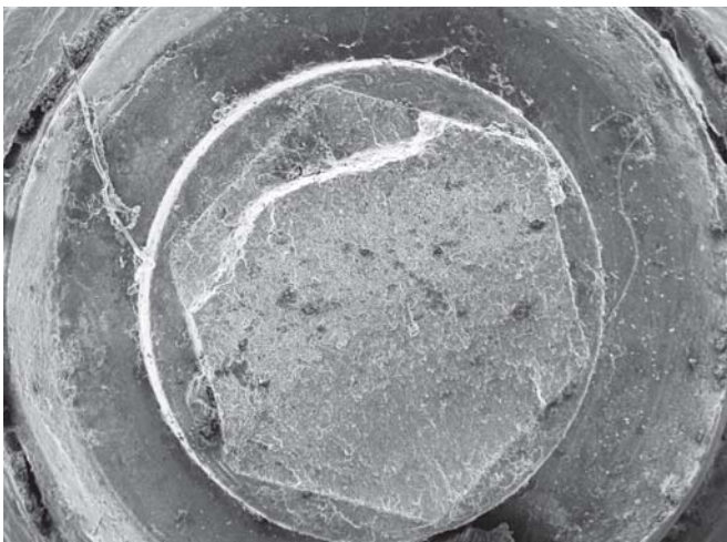
Fig. 5: SEM imaging (45x) of a crown prosthesis fractured at the fixture connection
