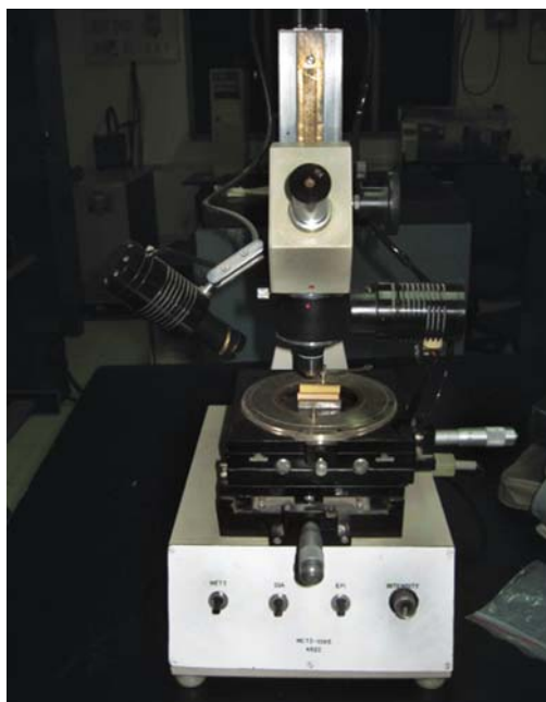
Fig. 7: Toolmaker's microscope (Metzer Opto Electrical Instruments Pvt Ltd, Bombay)
