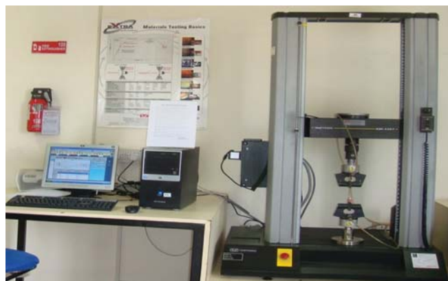
Fig. 8: Instron or Universal testing machine (Sintech 1123, Renew, Minneapolis, Minn)
