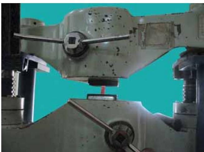
Fig. 5: Universal testing machine
