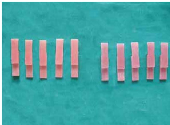
Fig. 4: Overlapping joint specimen
