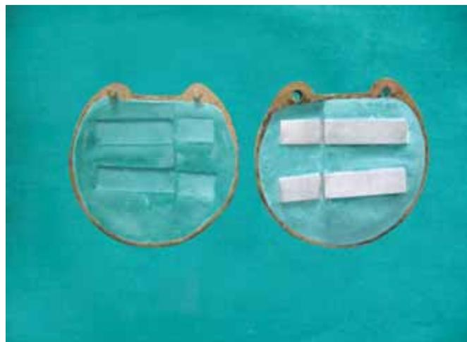
Fig. 3: Overlapping joint mold
