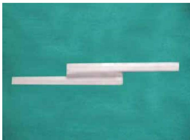
Fig. 2: Overlapping stainless steel joint specimen
