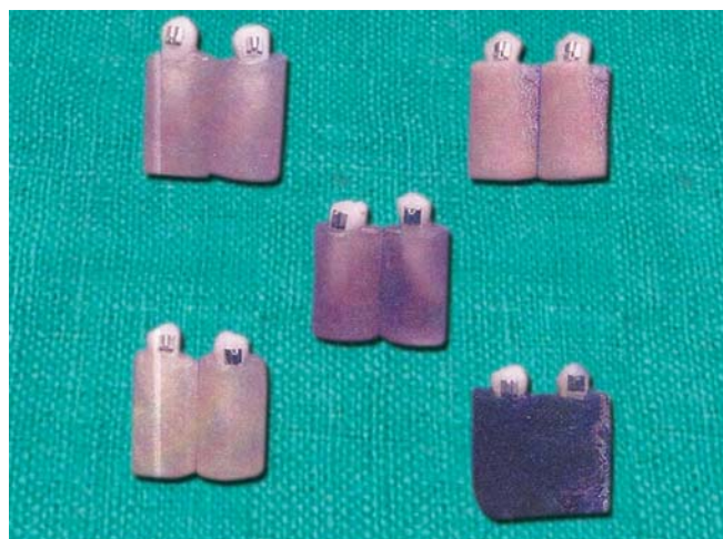
Fig. 3: Specimen bonded with the brackets
