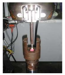
Fig. 8: The loading fixture with the specimen (Universal testing machine)
