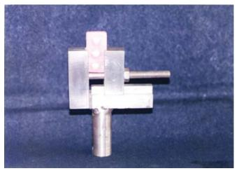
Fig. 4: Jig holding specimen
