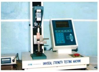
Fig. 5: Specimen being loaded
