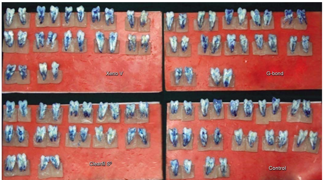
Fig. 1: Specimens after thermocycling and dye penetration
