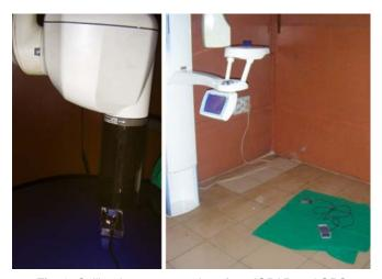
Fig. 1: Calibrating exposure dose from IOPAR and OPG machine using Unfors Mult-O-Meter
