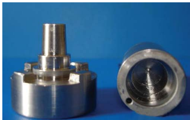
Fig. 2: Machined stainless steel master die analogs to a complete veneer crown preparation
