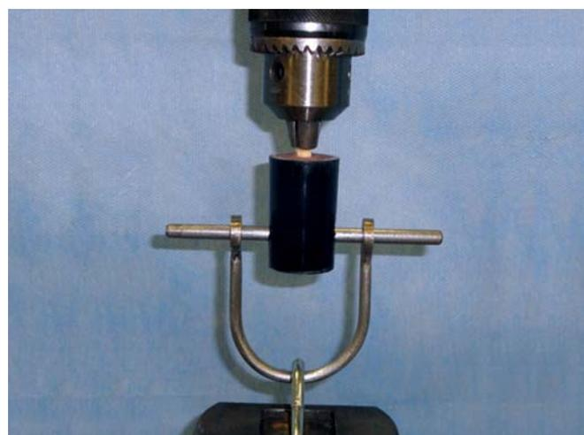
Fig. 1: Specimen mounted in Instron machine for bond strength test
