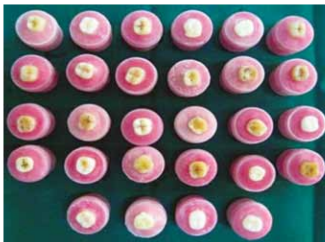
Fig. 1: Mounted samples in acrylic molds
