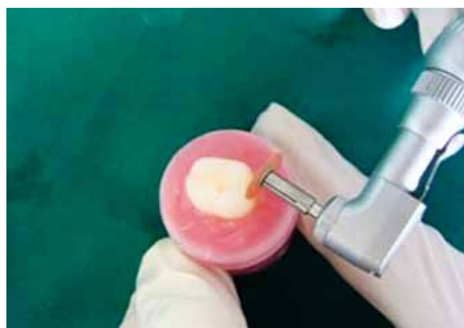
Fig. 2: Preparation of samples using silicon disks
