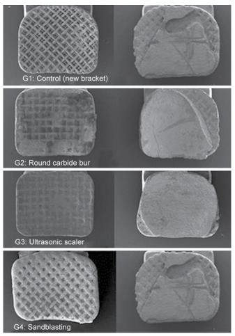
Fig. 1: SEM of the bracket bases of the different tested groups before bond up and after debond
