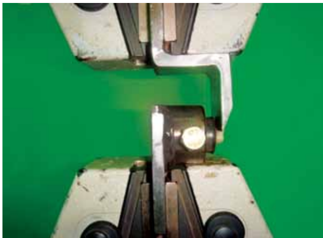
Fig. 4: Cured models subjected to shear failure loads on universal testing machine with the help of custom made jigs
