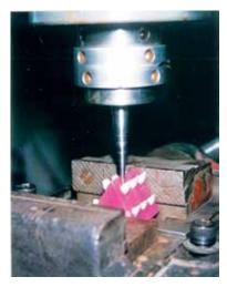
Fig. 7: Acrylized teeth with block fixed with grips for testing
