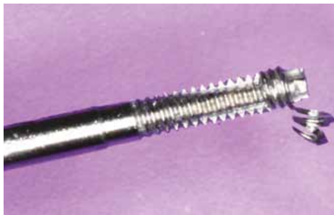
Fig. 8: Remaining fractured locator abutment screw fragment removed
