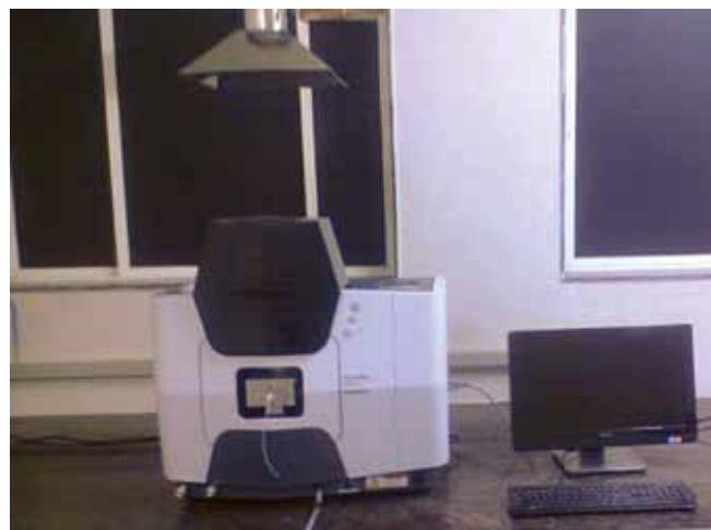
Fig. 5: Atomic absorption spectrometer (Shimadzu Model no. AA 7000, Maryland, North America)
