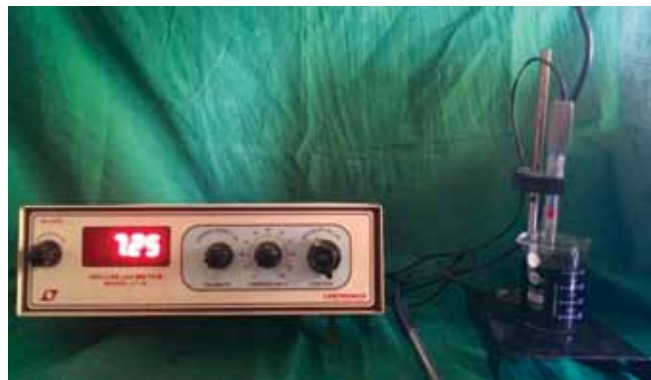
Fig. 3: Portable standard digital pH meter (Deluxe Labtronics LT 10, Haryana, India)
