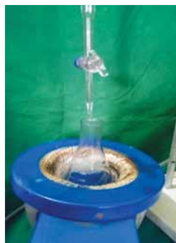
Fig. 2: Lane-Eynon test for sucrose estimation—titration of the Fehling's solution by the medicine sample in burette
