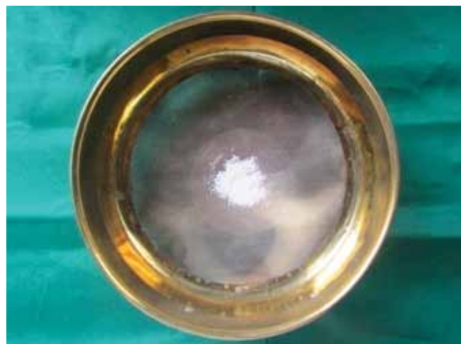
Fig. 4: Sieving the enamel powder through standard no. 85 mesh
