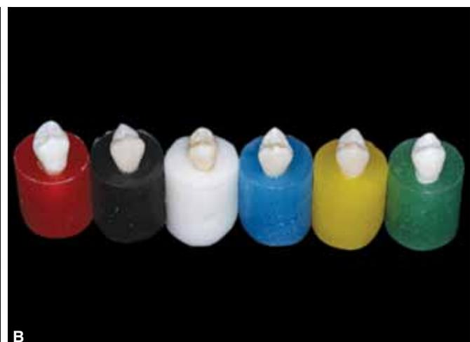
**Figs 1A and B:** (A) Teeth being mounted in a cylindrical base; (B) Teeth embedded in acrylic resin (each color indicates an experimental group)
