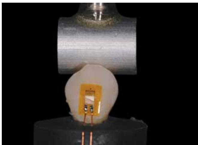
**Fig. 3:** Static compressive load applications on teeth
