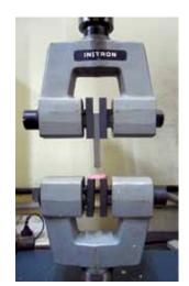
Fig. 1: Measurement of pushout bond strength using Instron Universal Testing Machine
