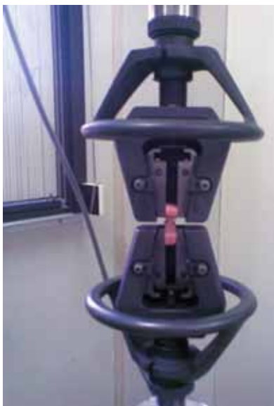
Fig. 2: The sample in position in the Instron testing machine
