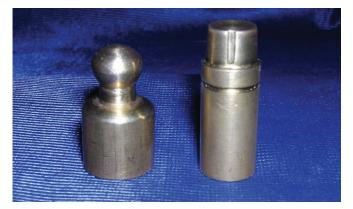
Fig. 1: Master model with counter die
