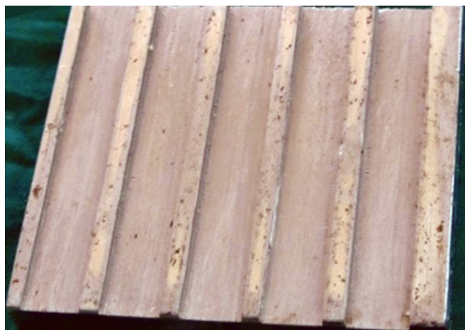
Fig. 1: Metal mold used for fabrication of wax patterns
