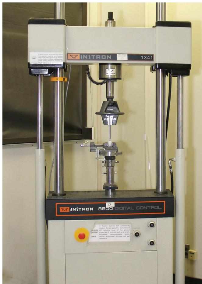
**Fig. 1:** The Instron machine used for testing. Note the specimen in place for testing the CS
