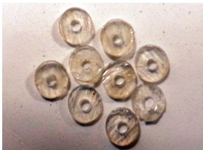
Fig. 2: Tygon tubings of internal diameter of 0.8 mm and height of approximately 0.5 mm
