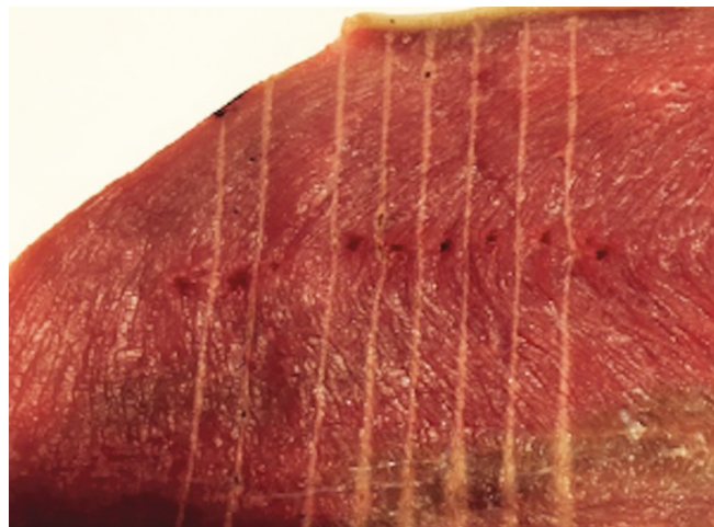
Fig. 3: Sample obtained after the irradiation, the holes are the site where thermocouples were positioned
