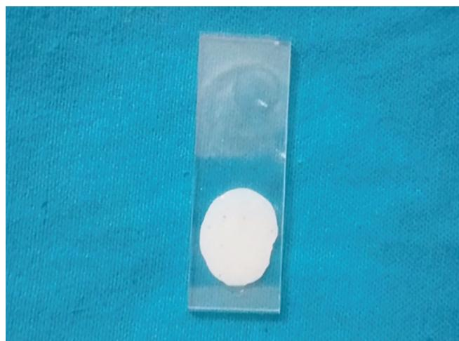
Fig. 2: Testing of film thickness with a layer of cement in between two glass slabs
