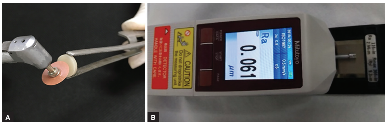
Figs 2A and B: (A) Finish and polish the specimens; and (B) evaluation of roughness using a roughness meter
